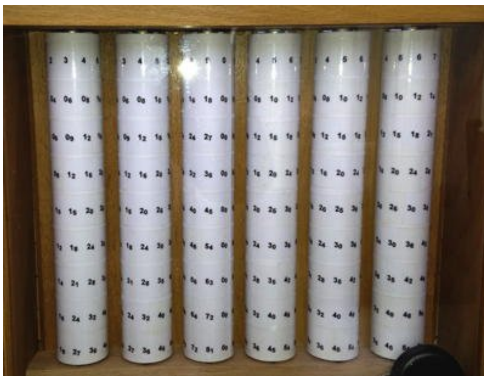
Figure 3.15. Schickard rear view showing Napier cylinders (collection Calculant)
