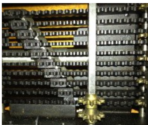
Figure 4.10. Rack mechanism of a Mercedes-Euklid 29 calculator. (collection Calculant)
