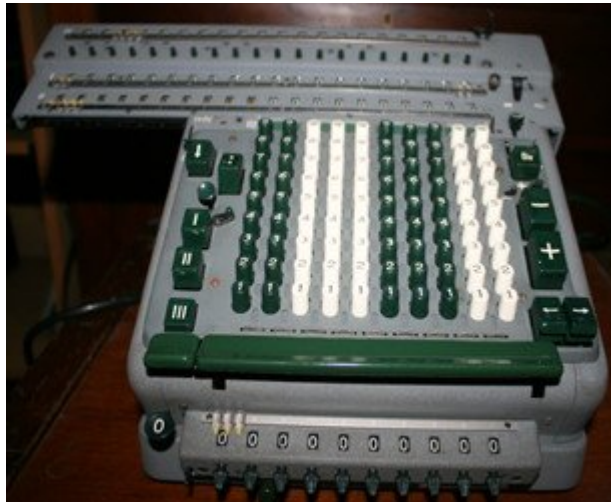
Figure 4.19. 1950s-1960s: MADAS Model 20BTG serial 94046 electric calculator with true automatic division (collection Calculant)
