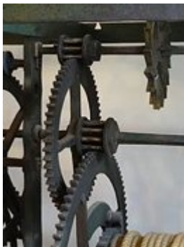
Turret clock with lantern gears 103 from 1608
