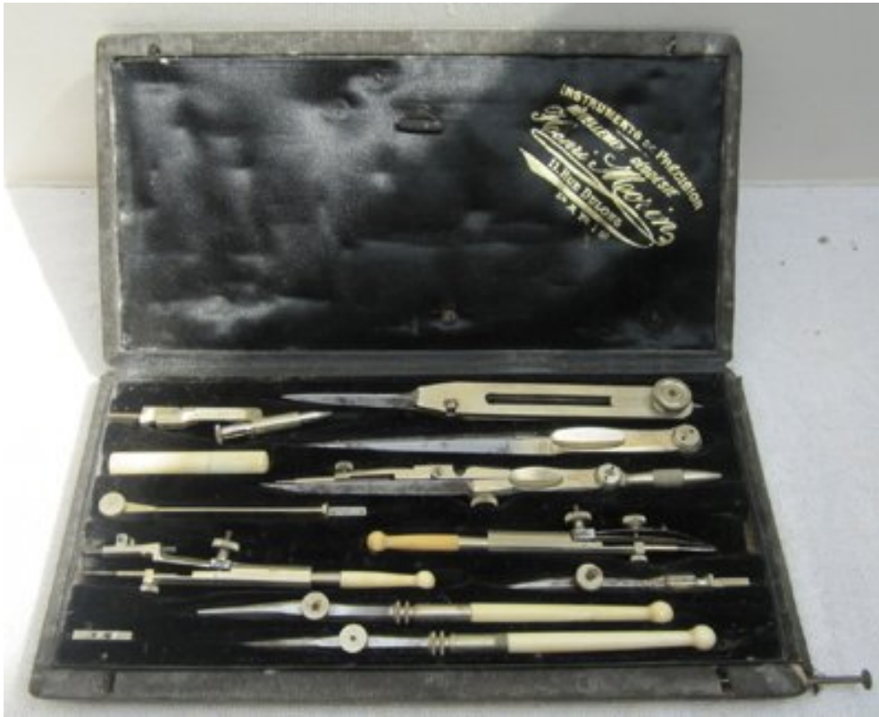
Figure 3.5. French drawing instruments ~1880 (including proportional dividers- top right) (collection Calculant)
