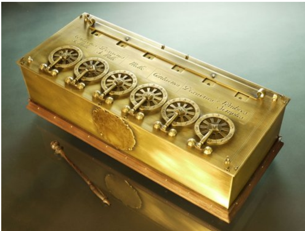
Figure 3.16. Working replica of a Pascaline, 98 style ~1650 (collection Calculant)
