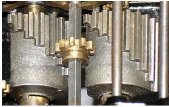
Figure 3.20. Twentieth Century step drum following the same principle as Leibniz's conception 134
