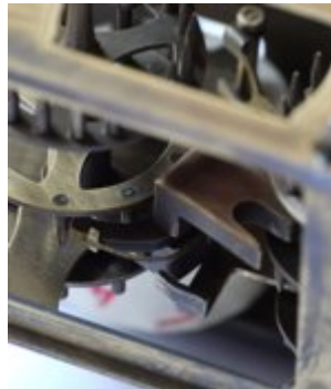
Replica fork-shaped carry mechanism (sautoir) (collection Calculant)
