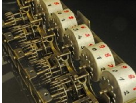
Replica Pascaline mechanism with spoked lantern gears (collection Calculant)
