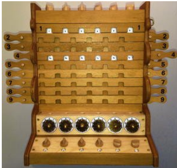
Figure 3.13. Working replica of Schickard's Calculating Clock (1623) (collection Calculant)
