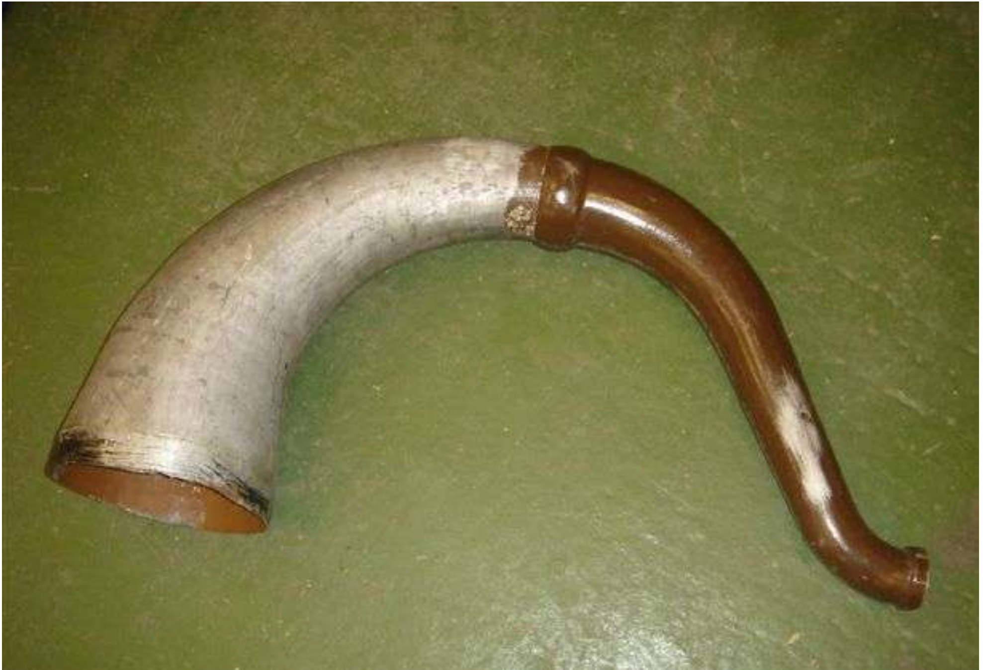
Mk Xb aluminium swan's neck horn casting---original.
