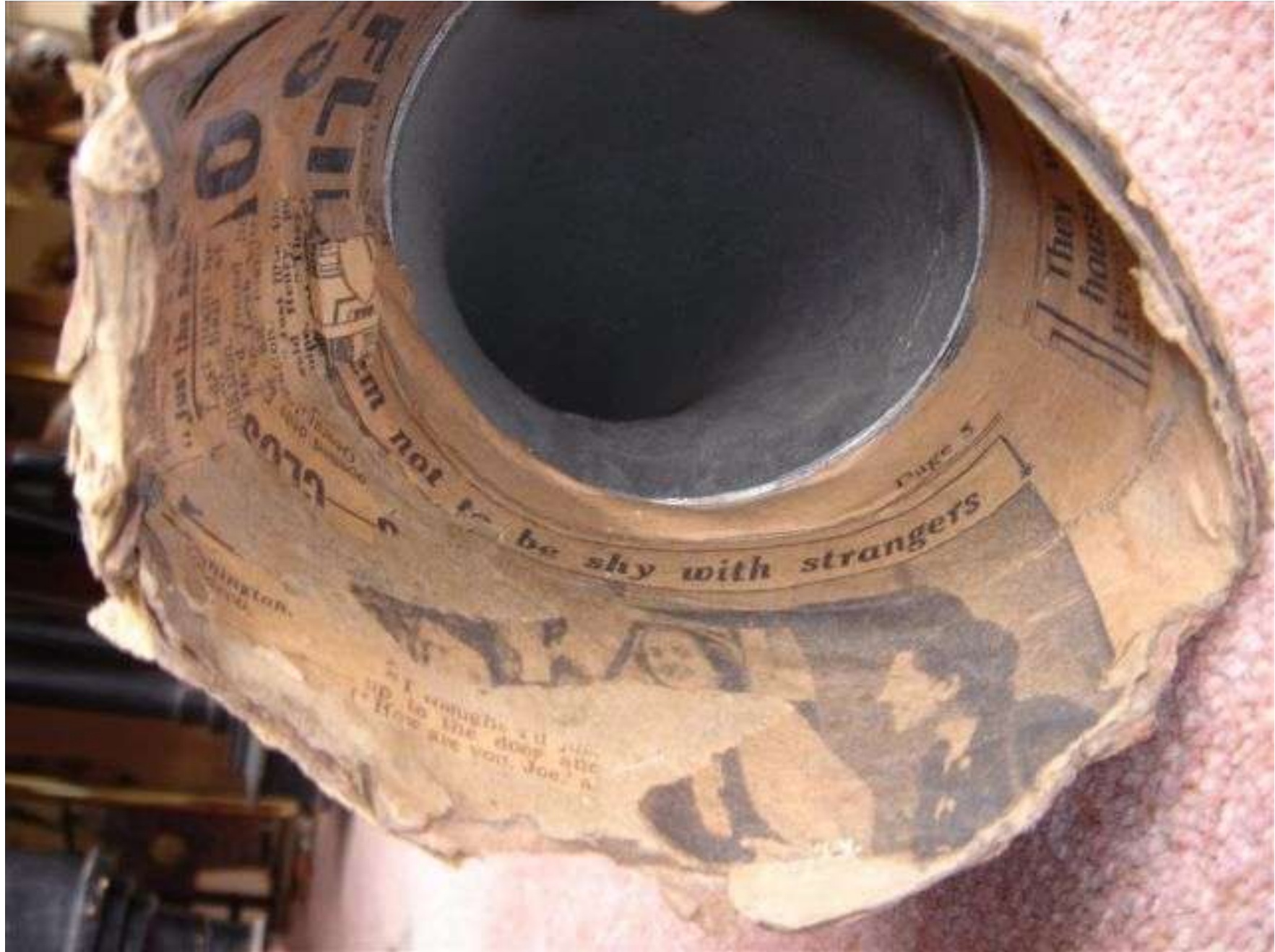
Mk IX horn showing page 5 girls and the other layers of paper which seem to be some sort of (quite thick) cardboard (some 22 thou') before the finishing paper.
